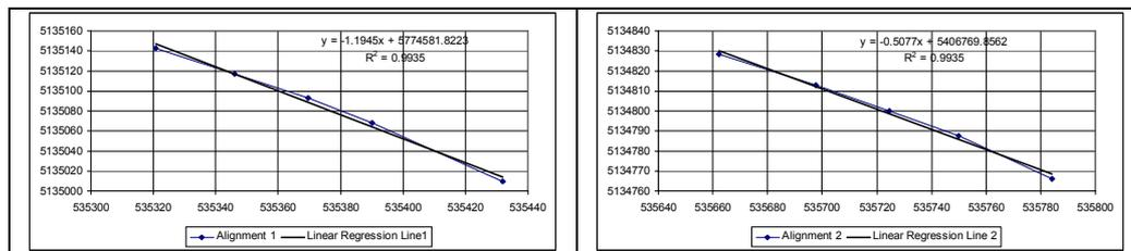
Figure 6. Horizontal alignment for two consecutive straight lines
