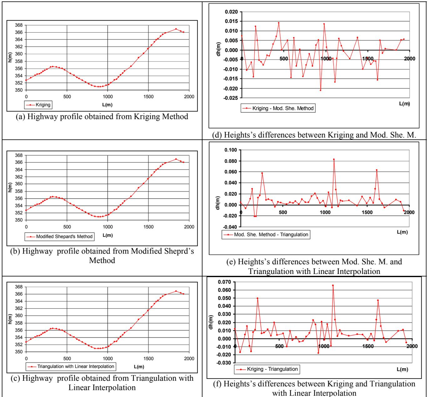
Figure 8. Profile sections via different digital elevation models and differences between them
