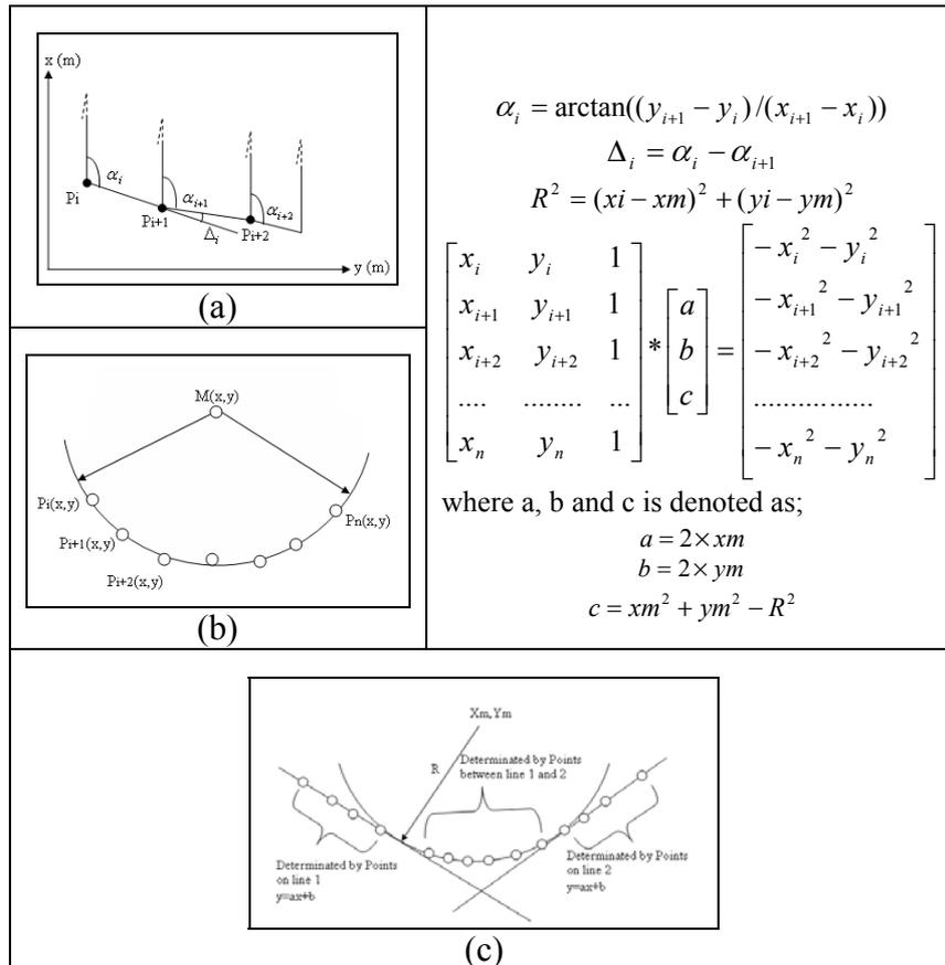
Figure 5. Evaluating horizontal highway geometry and its subsequent processes with equations
