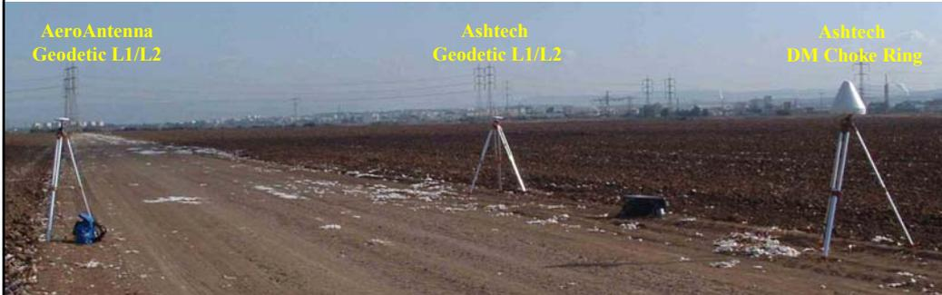
GPS day 301(2007), three GPS antenna types set up on a flat open field at a height of approx 1.6m.
