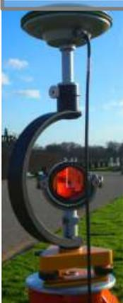
*Leica GRX1200GG Pro receiver with AX1202GG antenna operated with 20 Hz data rate*
