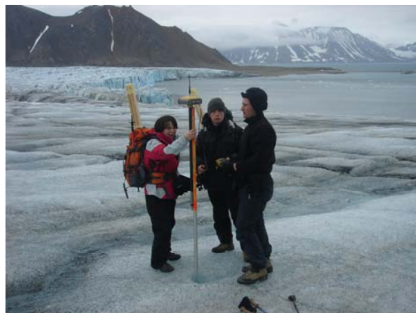
Fig.3. The progress of ablation staffs measurements by the RTK technique
