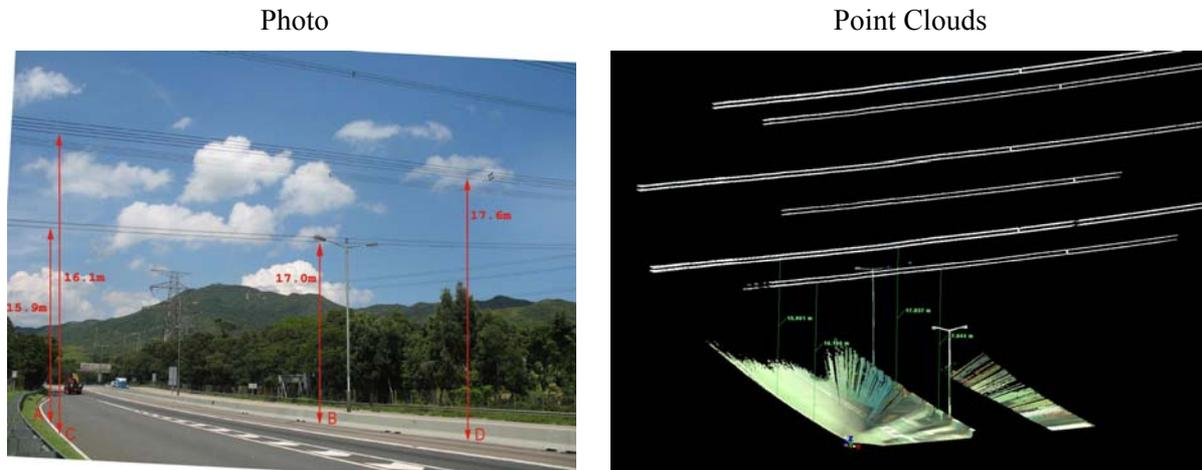
**Figure 5** – Photo and Scanned Point Clouds of Overhanging Cables across Fanling Highway
