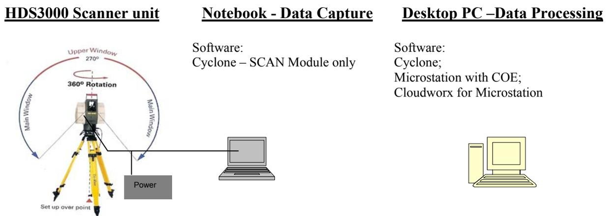
**Figure 1 – Setup of Terrestrial Laser Scanning System**
