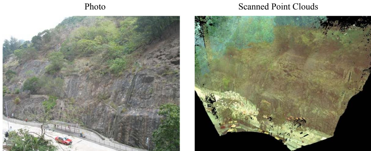
**Figure 3** – Photo and Scanned Point Clouds of Roadside Slope at Lin Tak Road
