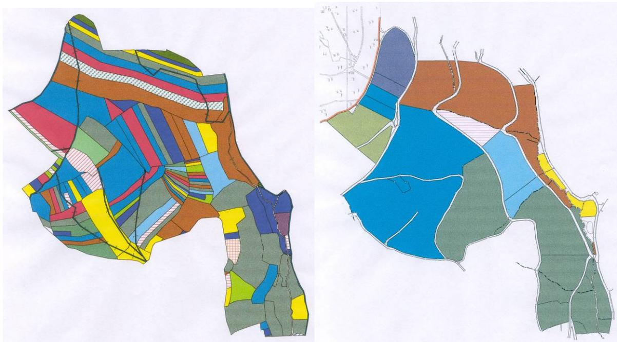
**Figure 5:** Extract of the ownership structure before (left) and after (right) the land consolidation Milchenbach
