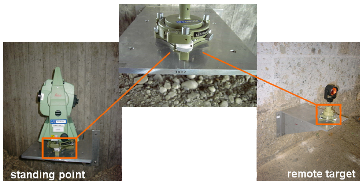
Fig. 5: Control network's core item: Mobile mounting panels with forced centering device
