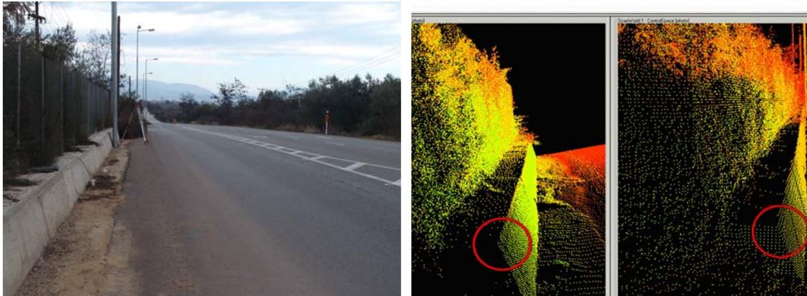
**Figure 5.** Spherical targets and homologous points
