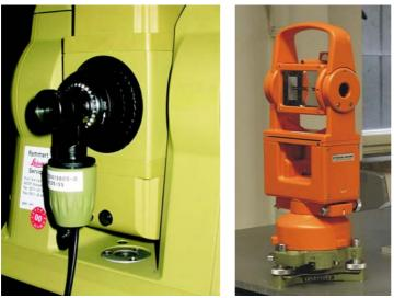
**Fig. 2:** Autocollimation-eyepiece from Leica Geosystems and Autocollimation-mirror GAP1 form Wild Heerbrugg.
