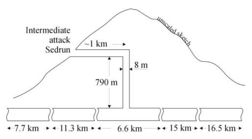
Fig. 1: Cross-section through the intermediate attack in Sedrun.
