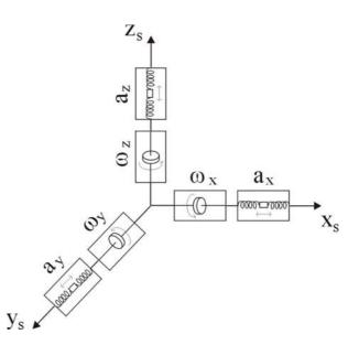
Fig. 3: Arrangement of sensor-axes of an IMU.
