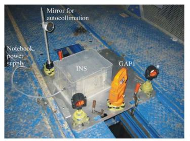
Fig. 4: mounted platform in the hoisting plant.
