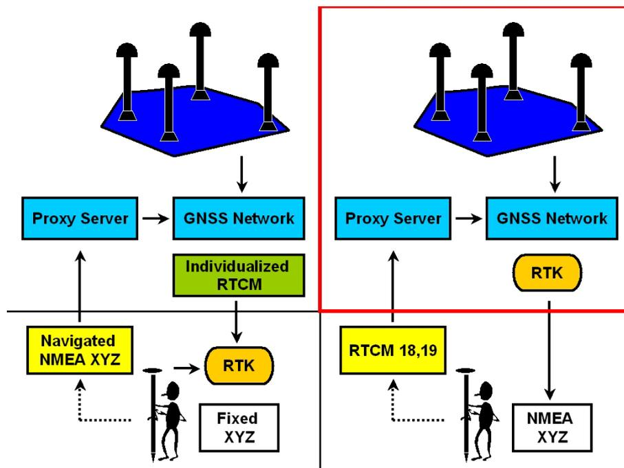
**Figure 1.** Standard GNSS-RTK (left), reverse (client-server) GNSS-RTK (right).
