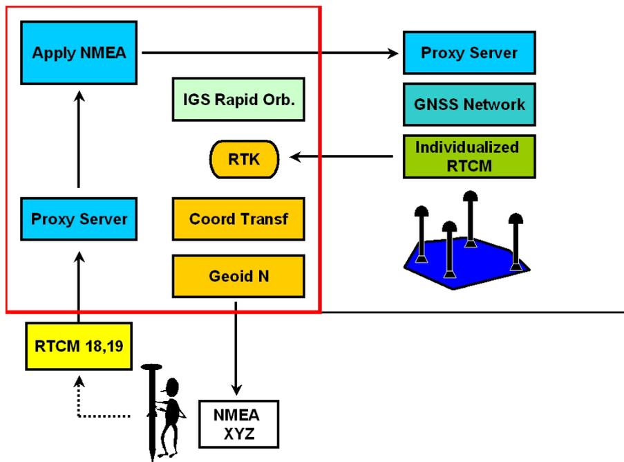
Figure 2. Sophisticated client-server GNSS-RTK model implemented transformations.
