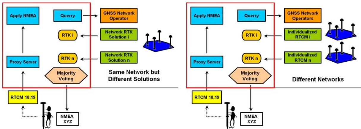
**Figure 3.** Concept of a GNSS service broker, accessing different DGPS services (left) or networks (right).
