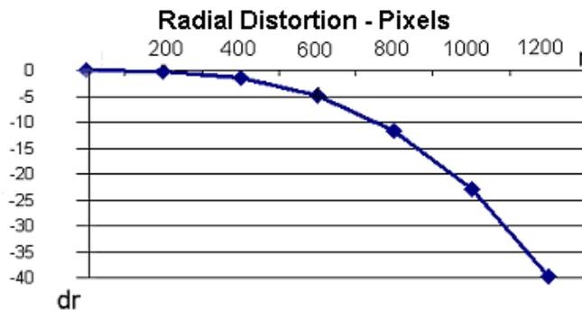
**Figure 1.** Curve of symmetrical radial distortion in pixels
