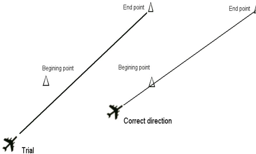
**Figure 8.** Procedure of navigation of flight route aiming at end point
