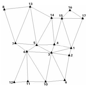
Figure 1. The 17-point GPS network
