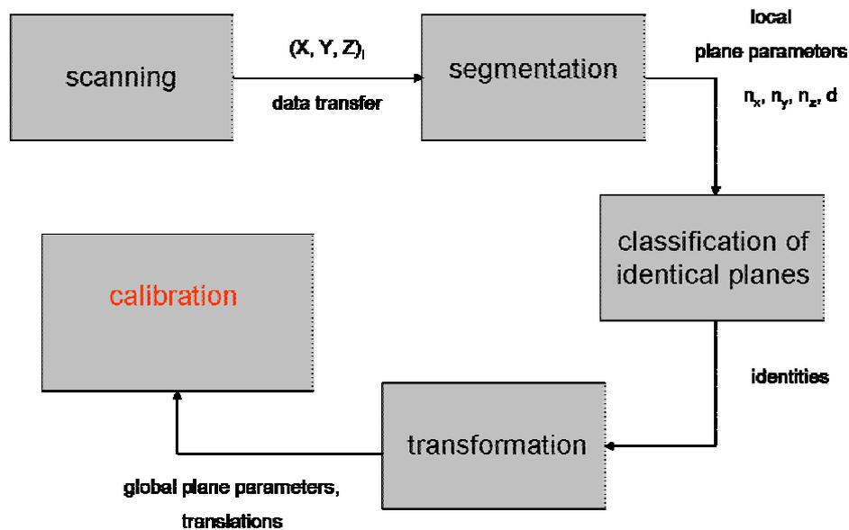
Fig. 4: Overview over the Calibration Procedure
