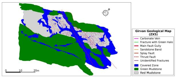
Fig. 3 Detailed map of the test area derived from the data of ZX5 representing the distribution and locations of the structural features (Tziavou, 2016)
