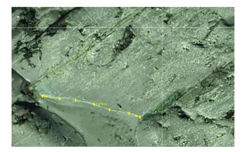
Fig. 5 The length of a joint could be specified with at a level of detail better than 1 cm. (Tziavou, 2016)
