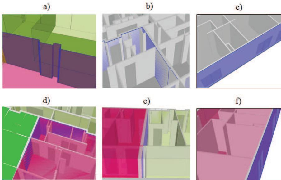
**Figure 9. Visualization of structural boundaries in BIM models: a) Visually ambiguous boundary type in legal model b) Internal boundary in physical model c) External boundary in physical model d) Internal boundary in integrated model e) Median boundary in integrated model f) External boundary in integrated model**
