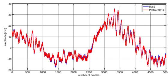
Fig. 15 Comparative measurement Profiler 9012 and IATS
