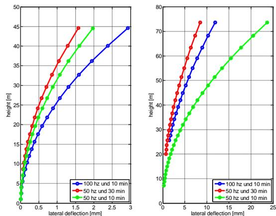
**Fig. 12 and Fig. 13** Bending lines TW600 and MM92
