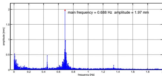
**Fig. 10** Amplitude spectrum of TW600 at a height of 44 m
