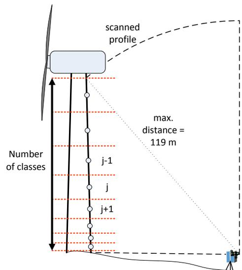
Fig. 6 Measurement configuration, side view
