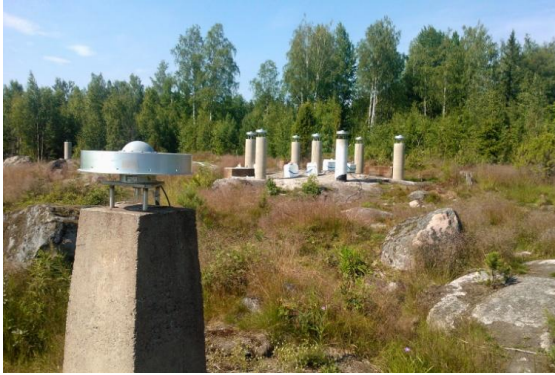
Fig. 3 Revolver test field for the verification of antenna calibration parameters at the geodetic fundamental station of Metsähovi, Finland.
