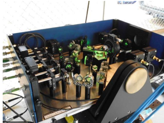
Fig. 1 TeleYAG measurement head mounted at the baseline.
