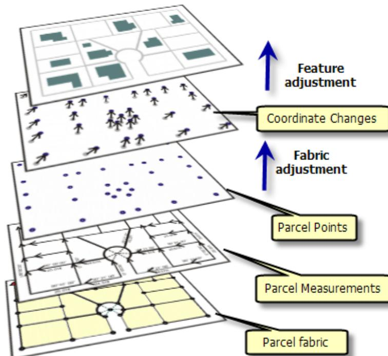
Figure 5. Feature adjustment based on parcel fabric adjustment
