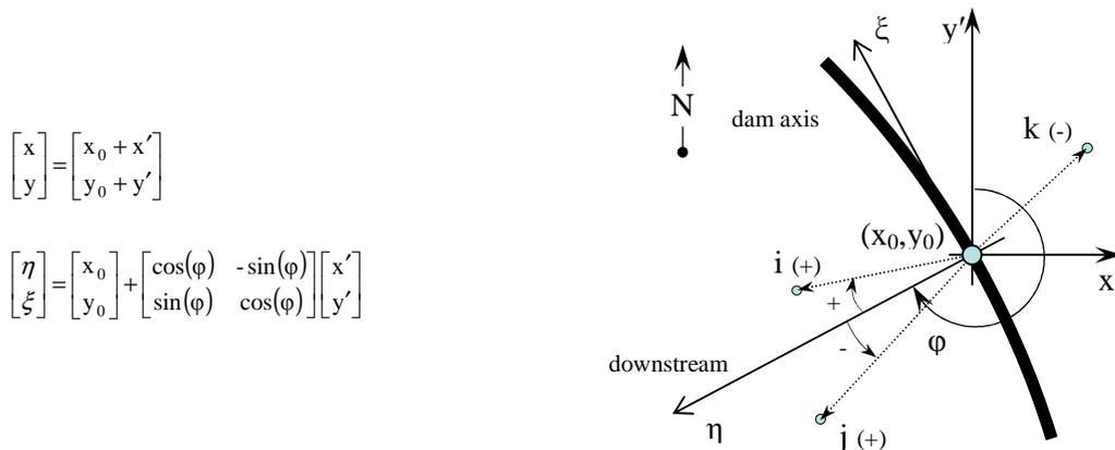
Figure 7 - Coordinate transformations of computed displacements. Deflections pointing downstream are positive (upstream negative).
