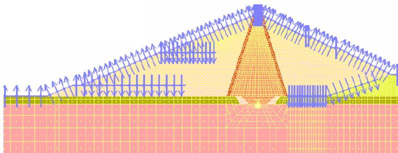
Figure 6 - Modeling of seepage forces
