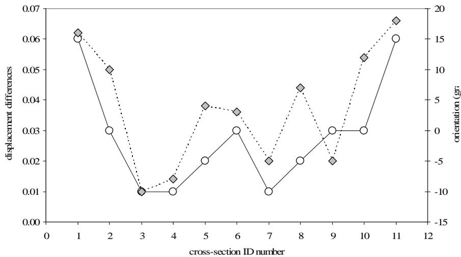
Figure 9 - Differences in the horizontal displacements computed for the eleven cross-section locations at the crest of the dam between geodetic monitoring and FE modeling (circles), and deviation in the orientation of the geodetically derived displacement vectors from the upstream-downstream direction (rhombs) for the period 1979-2005
