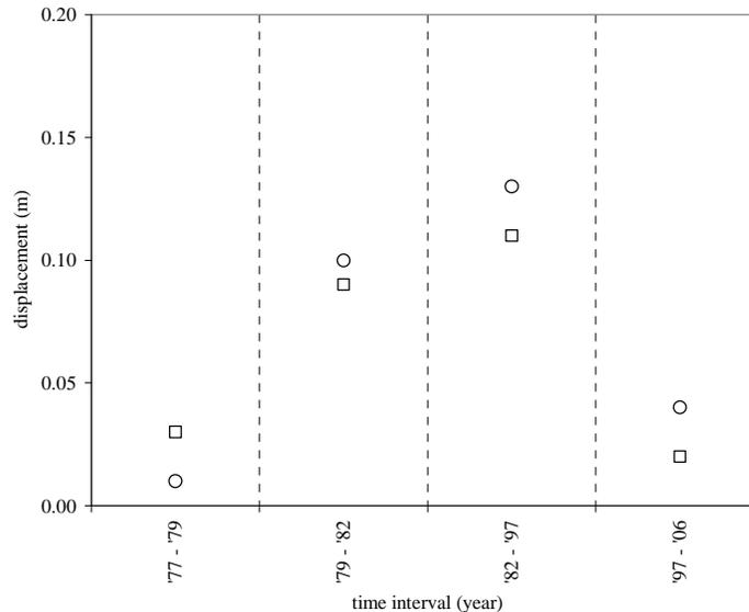
Figure 8 - Horizontal displacements ( $\eta$ -component) at cross-section 6 (middle of the dam) estimated by geodetic observations and FE modeling. The periods 1979-1982 and 1982-2006 correspond to the stages of first filling of the reservoir and operation of the dam
