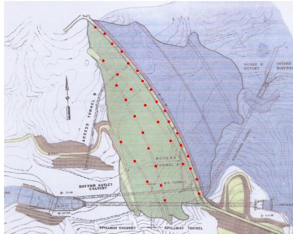
Figure 3- Geodetic control points at the crest and downstream abutment
