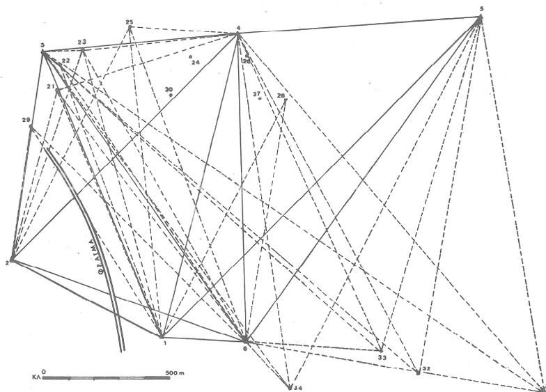
Figure 2 - Dam site and geodetic network
