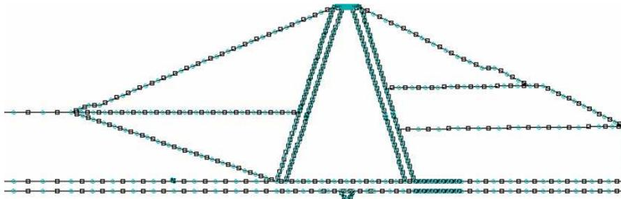
Figure 5 - Construction of FE mesh
