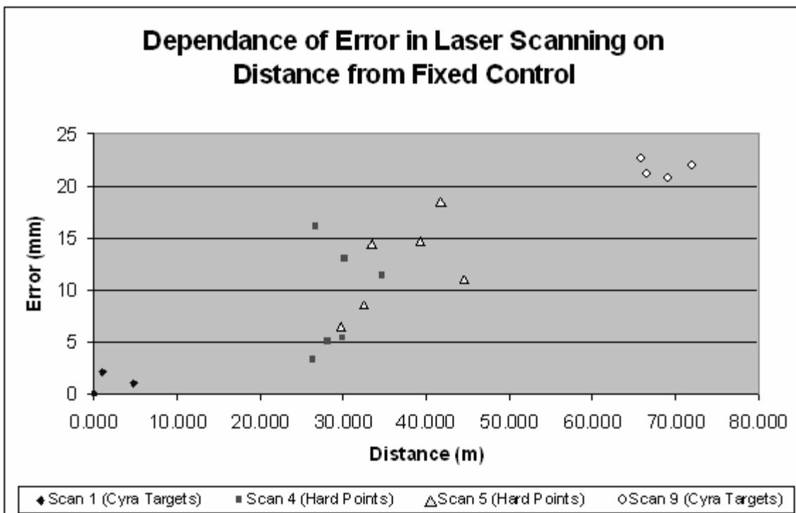
**Figure 5:** 3D Error vs. Distance
