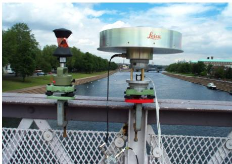
Figure 2 The total station 360° prism located next to the GPS antenna
