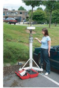
Figure 6 The GPS antenna and the total station prism housed together as one unit on a monument
