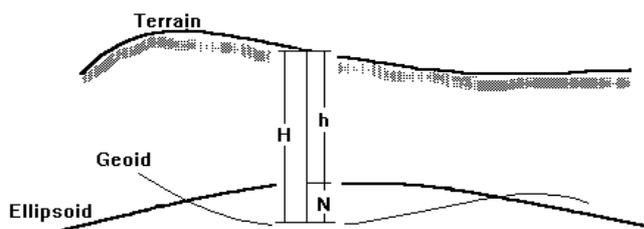
Fig.2 The definition of the two height systems in Geodesy
