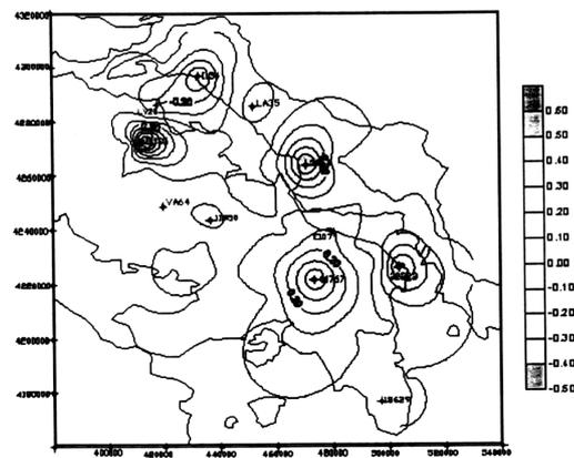
Fig. 4 Kriging interpolation errors with trend of EGM96 truncated at n=90
