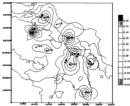
Fig. 3 The linear interpolation errors with trend of OSU91A truncated at n=90
