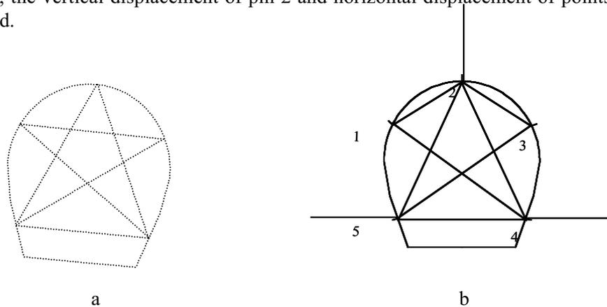
Figure 4: Finding deformed profile (a) and measurement of total tunnel displacement at three points (b).
