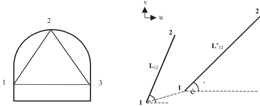
Figure 6: Length change after moving two points of a diagonal.
