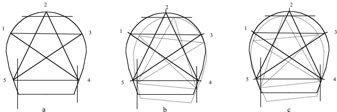
Figure 5: Finding the final shape of the deformed profile graphically.
