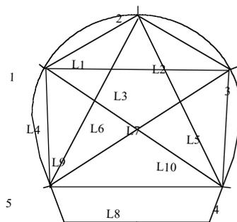
Figure 1: Possible diagonal readings with 5 pins.
