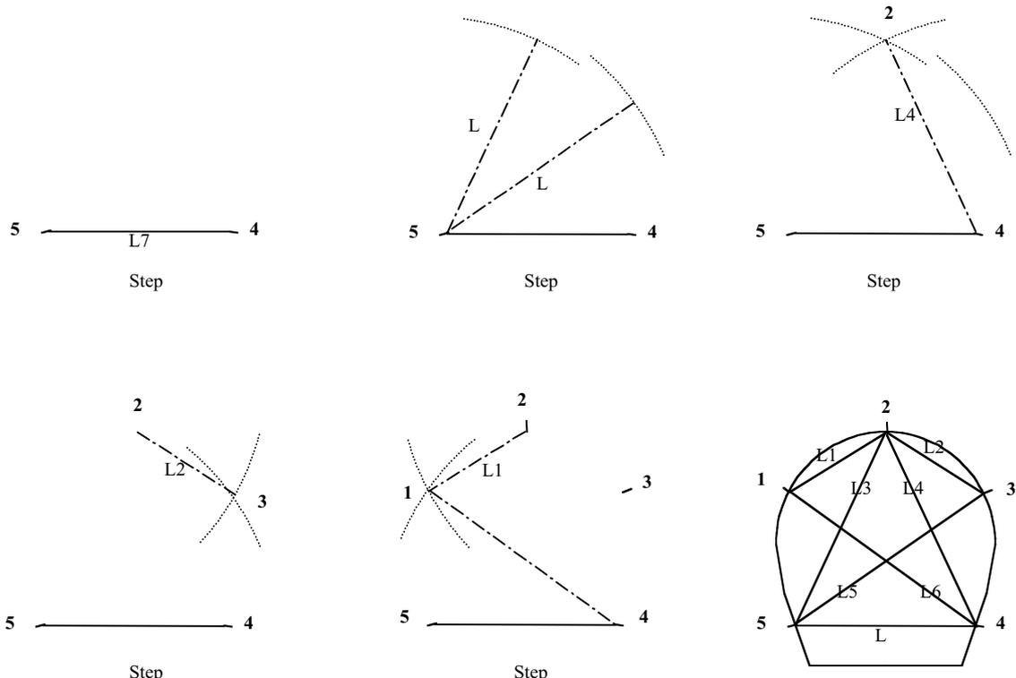
Figure 3: Steps for finding the coordinates of pins in graphical method.
