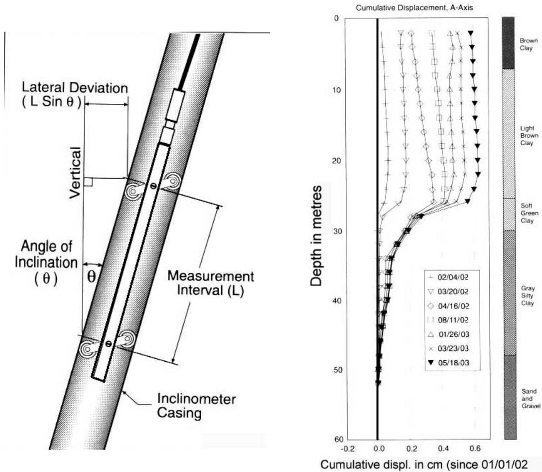
Fig. 6 : Left : Inclinometer probe and Right : typical horizontal displacement profile obtained by an inclinometer.
