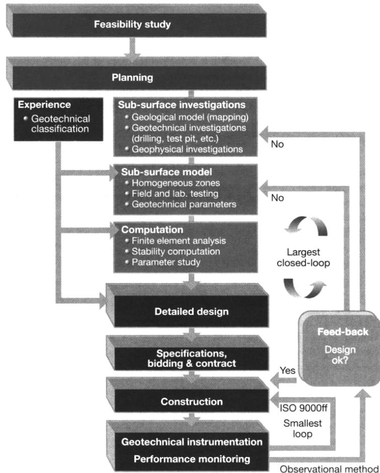
Fig. 2 : Deformation monitoring as part of the integrated design-construction-performance monitoring sequence. The smallest loop is used to adapt construction to the in-situ conditions. The largest loops are used to modify the design (sub-surface model) or even to require additional geotechnical investigations.
