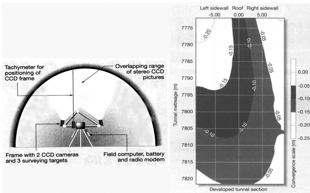
Fig. 3 : Typical features of the DIBIT tunnel profilometer (left) and typical plot of the measured wall convergence as contours on the developed tunnel wall area (Tunnels and Tunnelling, April 2001) .
