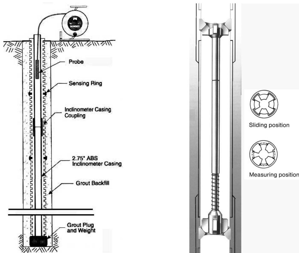
Fig. 5 : Left : Magnetic extensometer and Right : Fixed re-Installable Micrometer (FIM) of the Sliding Micrometer class, for in-depth vertical settlement measurements.
