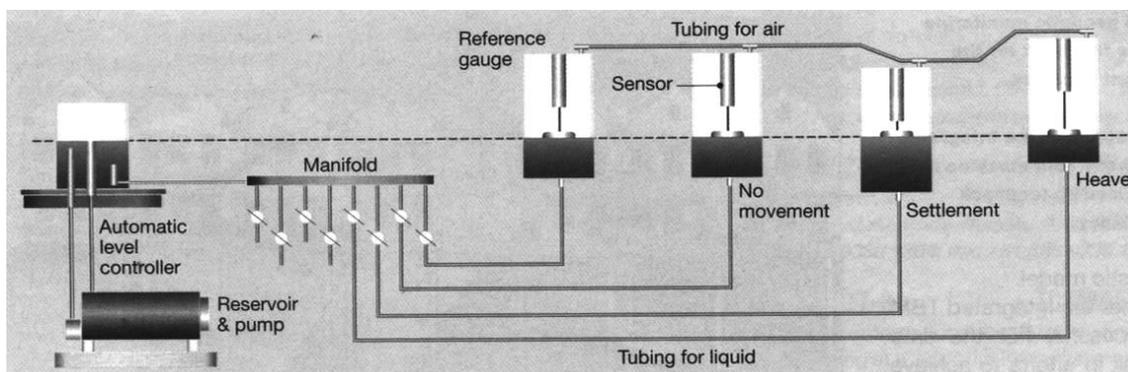
Fig. 9 : Electronic Liquid level gauge for measurement of settlements in several locations (after Tunnels and Tunnelling, May 2001)
