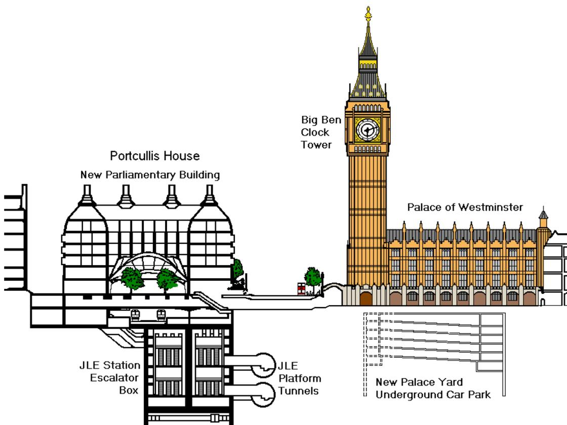
Fig. 10 : Cross section of the platform tunnels and the underground Westminster Station next to the Big Ben Clock Tower (after Burland et al, 2001).
