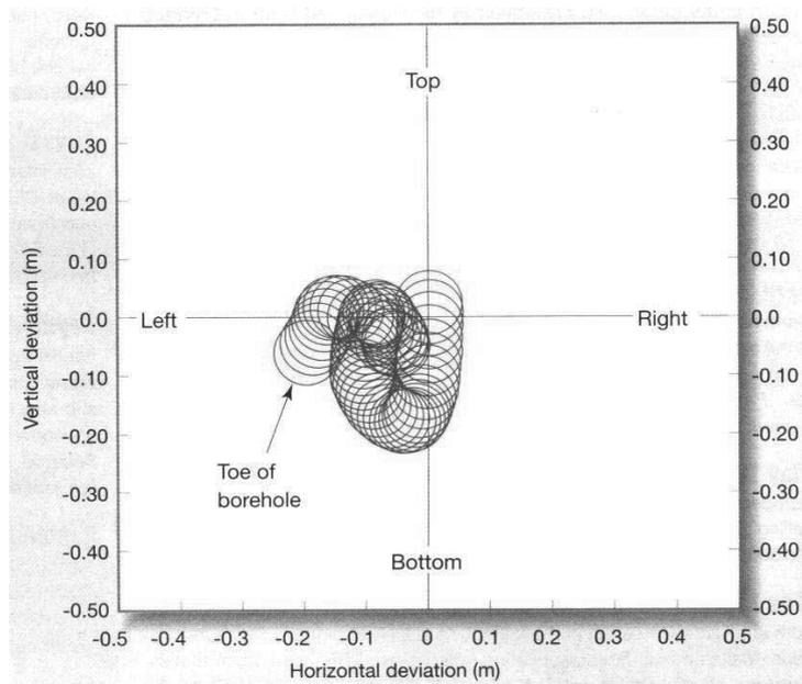
Fig. 8 : Application of the curve deflectometer in measuring the deviation of borehole alignment
