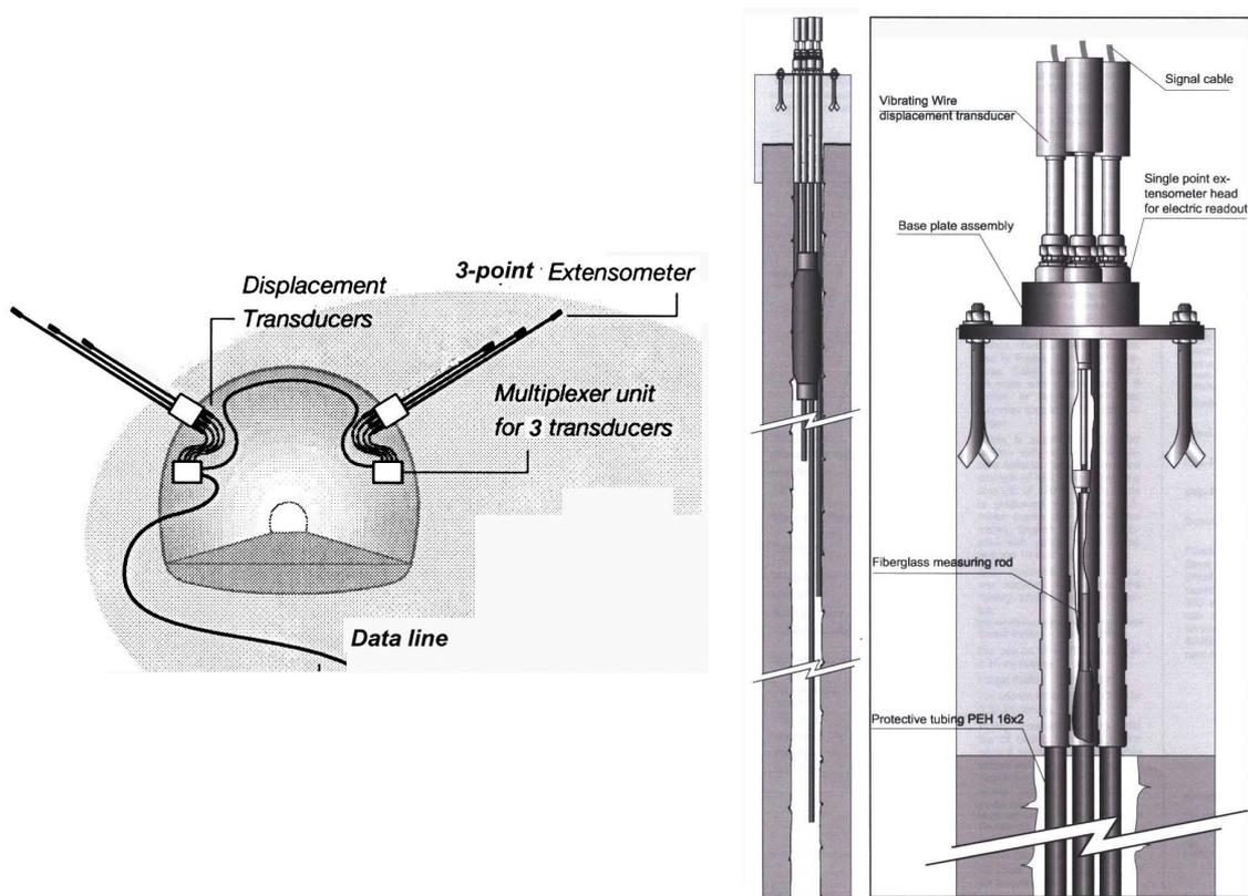
Fig. 4. Left : Three-point rod extensometers installed in boreholes drilled from the tunnel wall. Right : Detail of the measuring head of the instrument, using electronic displacement transducers for automatic recording of the measurements.
