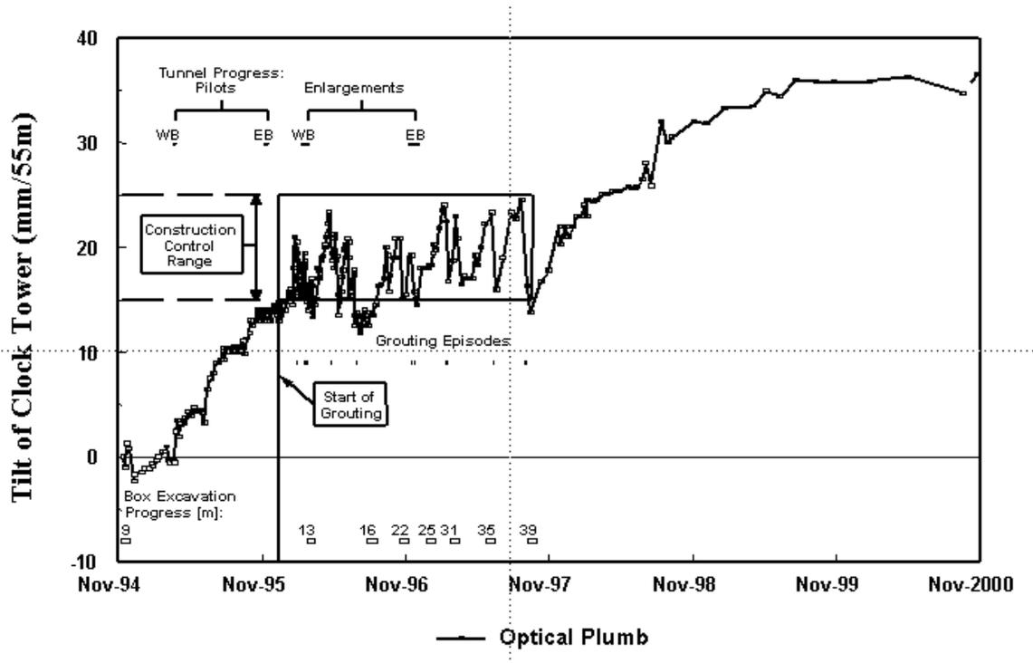
Fig. 11 : Monitoring of the tilt of the Big Ben Clock Tower (in millimeters of horizontal movement at the top of the 55m high tower) during the period of tunnelling and subsequent consolidation of the London Clay (after Burland et al, 2001).
