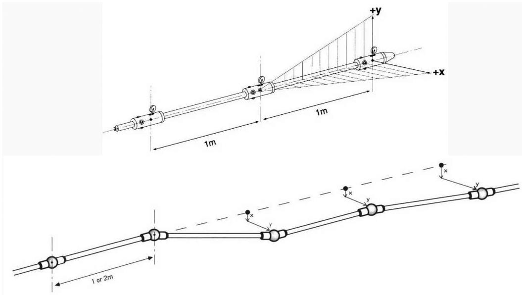
Fig. 7 : Top : Sliding curvometer and bottom : Chain deflectometer, for measuring deflections of boreholes in any orientation.
