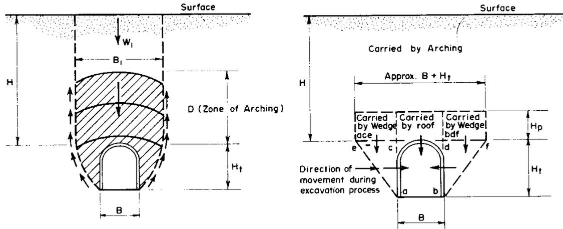
Fig. 1 : Terzaghi's recommendations for the loading on tunnel linings :
