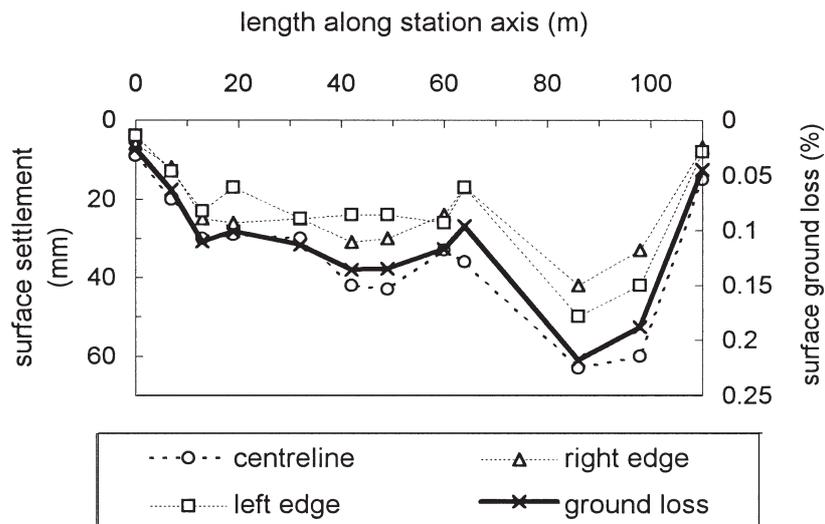
Fig. 13 : Measured ground surface settlements and ground loss factors along Omonia Station (after Kavvadas, 1998).
