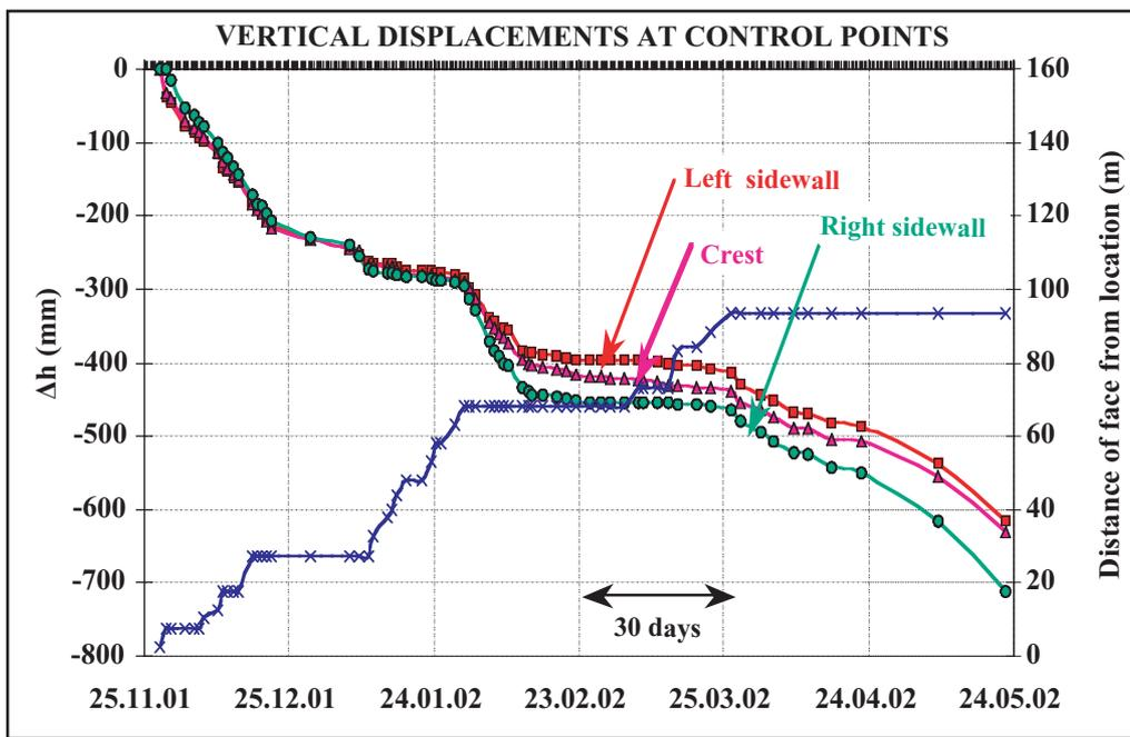
Fig. 15 : Monitoring of wall deformation (settlement) in a mountain tunnel. The abrupt increase of settlement after a period of apparent stabilisation indicates failure of the tunnel invert. After two consecutive such failures and repairs, the tunnel failed completely as shown by the abrupt increase of settlement at the end of May 2002.
