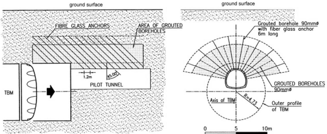
Fig. 12 : Ground pre-treatment with Tube-a-Manchette grouting from a pilot tunnel ahead of the tunnel face in the Athens Metro. Such ground improvement proved to be very effective in drastically reducing ground settlements and was used extensively in the Syntagma-Acropolis interstation where the tunnel passed below buildings of the Old City (Plaka) (after Kavvadas, 1999).
