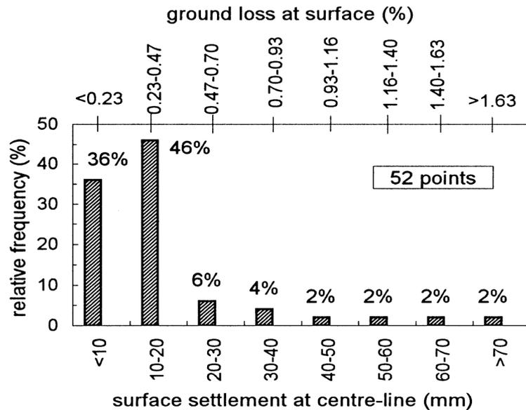
Fig. 14 : Statistical data of ground surface settlements due to TBM tunnelling in the Athens Metro Lines 2 & 3 (after Kavvadas, 1999).
