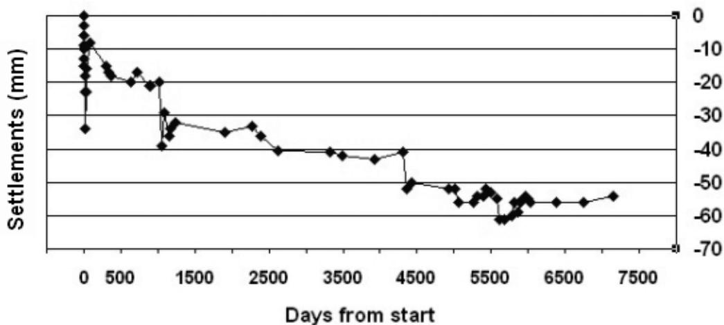
Fig. 8. Mean settlements of benchmarks R1, R2, ..., R8 for each epoch (1983 – 2003)
