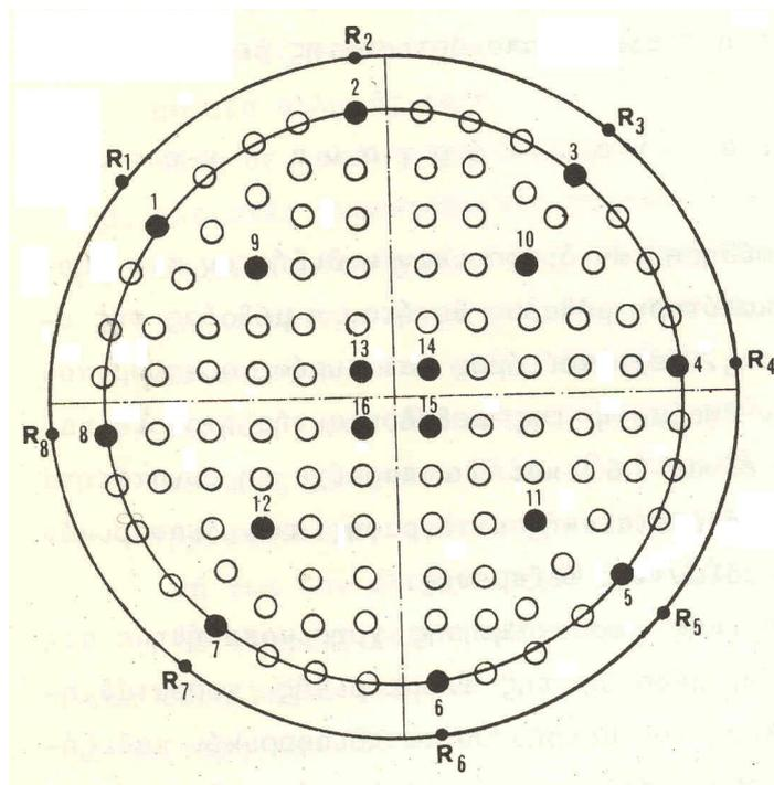
Fig. 2. Layout of the group of piles (black dots show piles with benchmarks for settlement monitoring)
