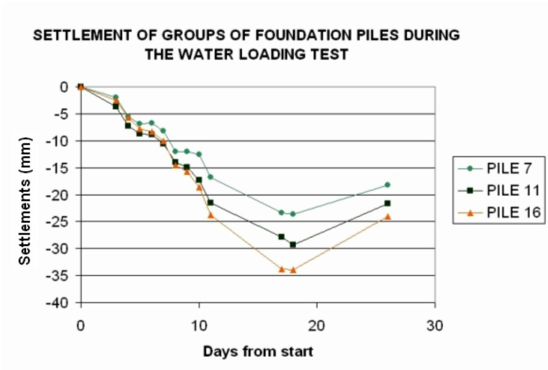
Fig. 5. Settlement of pile 7 (external periphery of slab), 11 (intermediate periphery), and 16 (center of slab)
