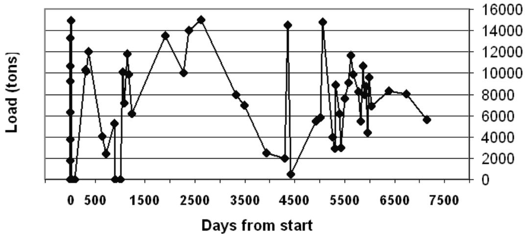
Fig. 7. Total loading history of the liquid ammonia storage tank (1983 – 2003)
