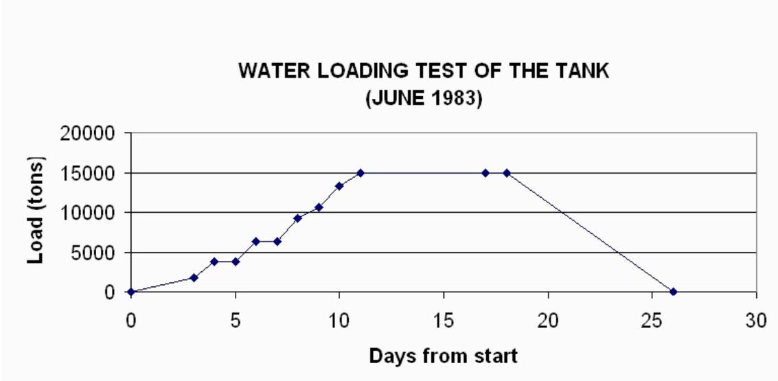
Fig. 3. The water loading test of the liquid ammonia tank in June, 1983
