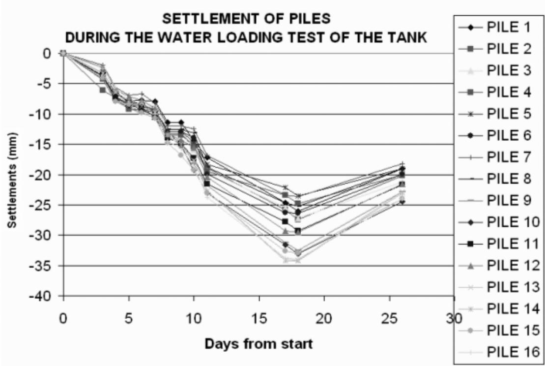
Fig. 4. Settlements of all piles during the water loading test of the tank in June, 1983
