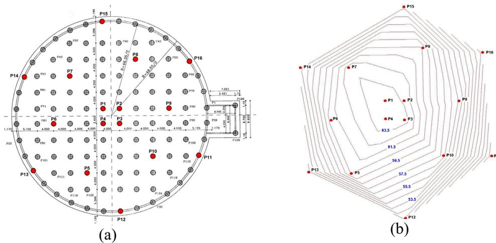
Fig. 9. Layout of foundation piles (a) and measured vertical displacements (b) of the 50,000 t sugar storage tank at Plati
