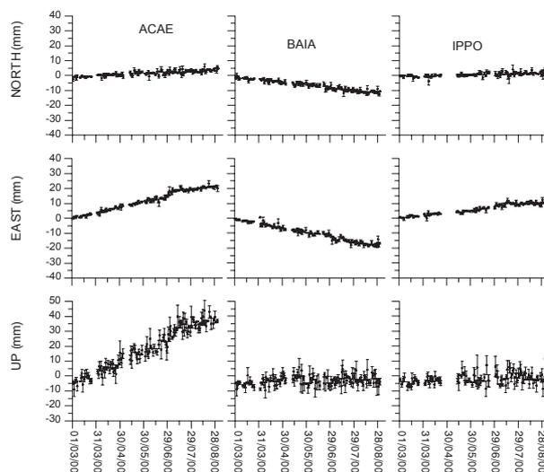
Fig. 13- Time variations of components for three baseline located in Campi Flegrei area, during the 2000 uplift episode
