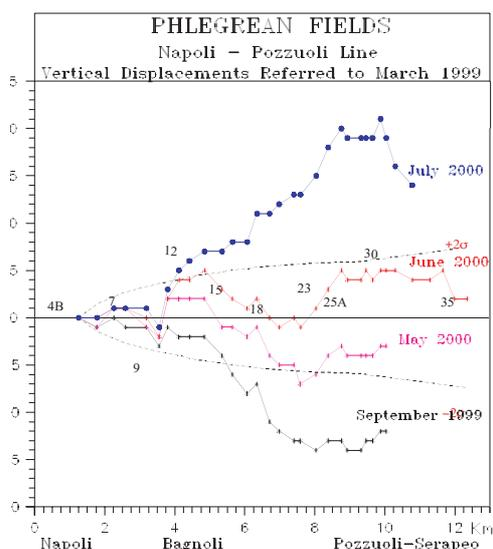
Fig. 12- Vertical displacements calculated during 2000 at Campi Flegrei, along the E-W line, as referred to March 1999 survey.
