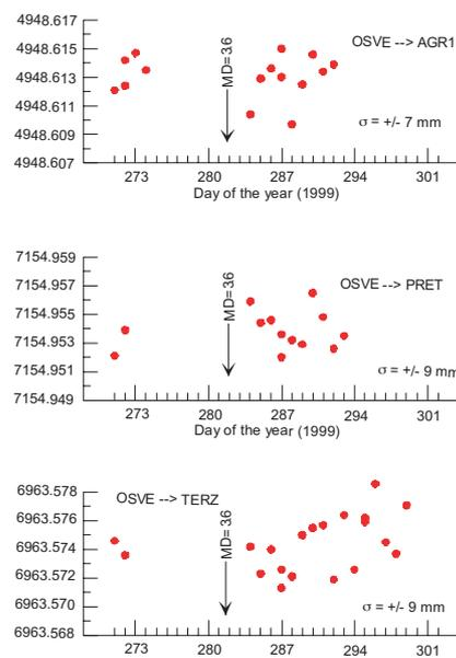
Fig. 6- Variation of the lengths for three baseline measured before and after the earthquake.
