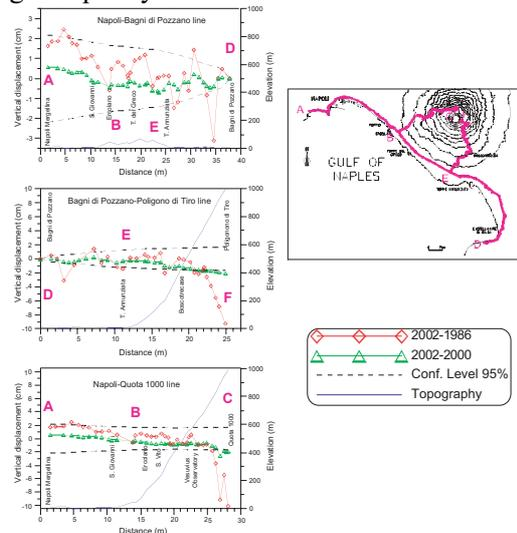
Fig. 3- Vertical displacements calculated on some circuits of the Vesuvius levelling network in the period 1986-2002. The location of lines is also reported.
