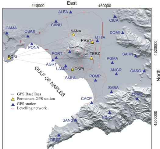
Fig. 2- GPS and levelling networks operating at the Vesuvius area.
