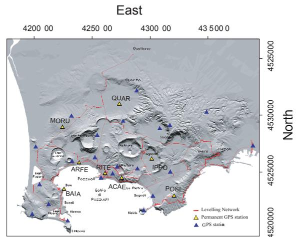
Fig. 9- GPS and levelling networks operating on Campi Flegrei.
