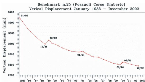
Fig. 8- Vertical displacements vs time at benchmark 25, located near to maximum uplift area, during the period 1985-2002.
