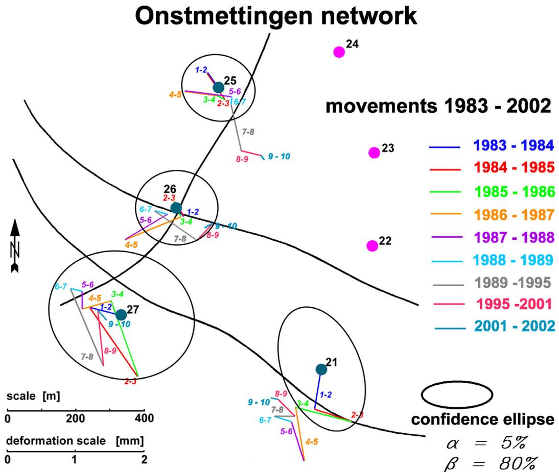
Fig. 5: Results of deformation analysis in the Onstmettingen network. A series of deformation vectors from epoch to epoch identifies the changes taken place. The confidence ellipses give a critical value the deformation can be evaluated to be significant. The scale of confidence ellipses is in accordance to the deformation scale.
