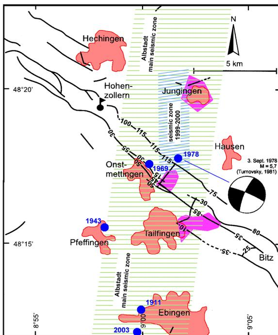
Fig. 1: Structure of Hohenzollerngraben, fault heights and location of the major seismic events and the established geodetic networks.
