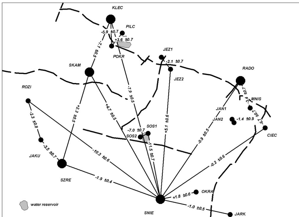
Fig. 6 The relative changes of selected vectors' length in years 2001-2002 (in mm).
