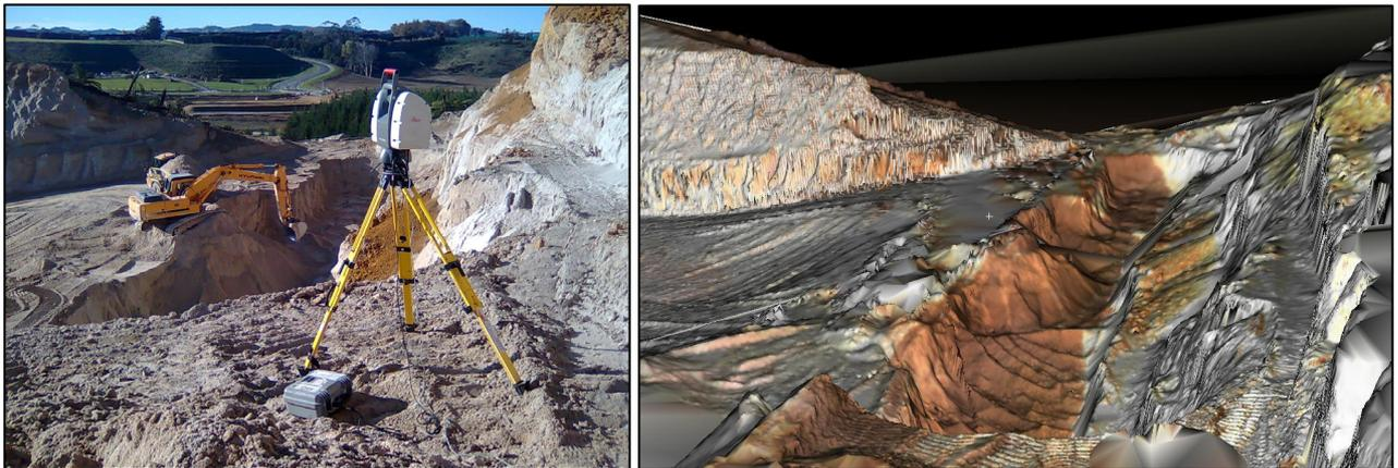
Scanning in operation during the excavation of one of the areas, and the resulting ground model (decimated)
