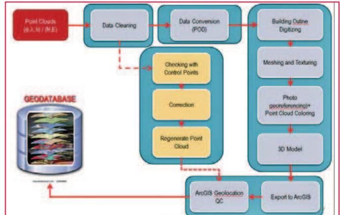
Figure 4: MTLs data processing methodology
