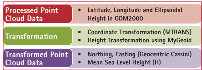
Figure 3: Coordinate Transformation for Point Clouds Data
