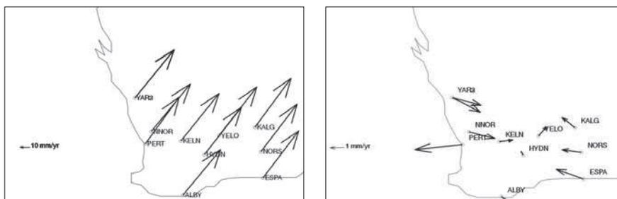
Figure 4: Absolute (left) and relative (compared to mean, right) velocities derived from combination of the individual GA and CUT APREF solutions using Bernese GPS Software version 5.
