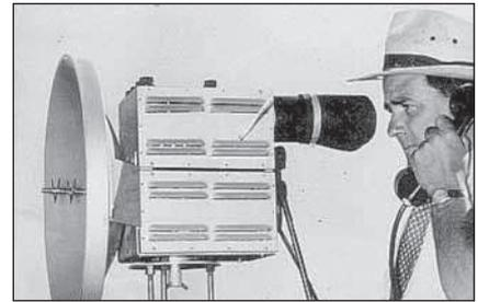
Dr Wadley with the prototype Tellurometer
