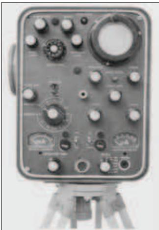
The control panel of the MRA2 Tellurometer
