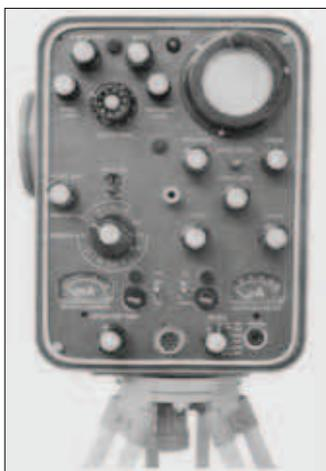
The control panel of the MRA2 Tellurometer
