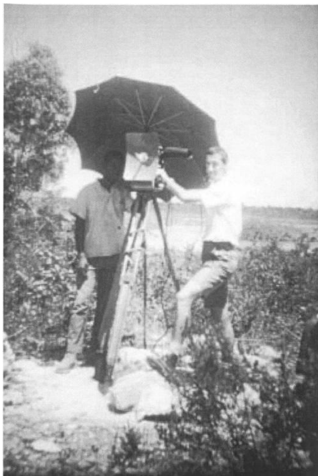
New Providence Island, Bahamas, September 1963. David Broome, chainman and Tellurometer MRA2. (See also colour page 20).
