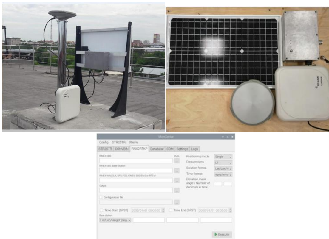
Figure 2: Elements of the cost-effective geodetic monitoring system
