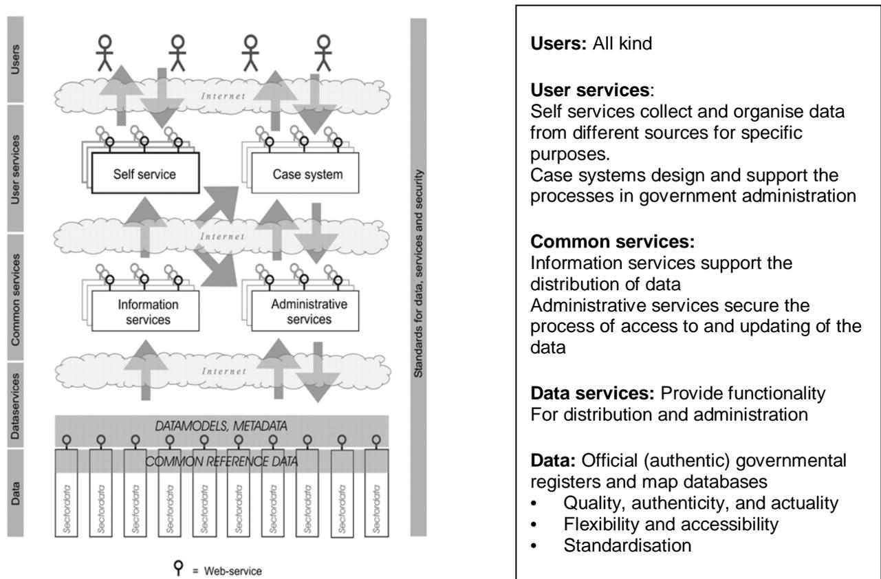
Fig. 3. The Danish concept for service-oriented IT-architecture.
