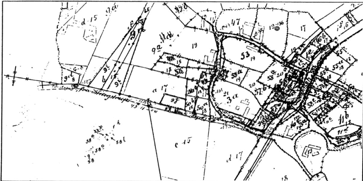
**Figure 5.** Part of an analogue cadastral map from 1983 as used, rectified, and updated over a period of about 100 years. The map is an “island map” and is not linked to a national grid. The display is difficult to interpret, and even though the map was redrawn in 1984, it is not efficient for daily land management. (Courtesy of the National Survey and Cadastre, Denmark).
