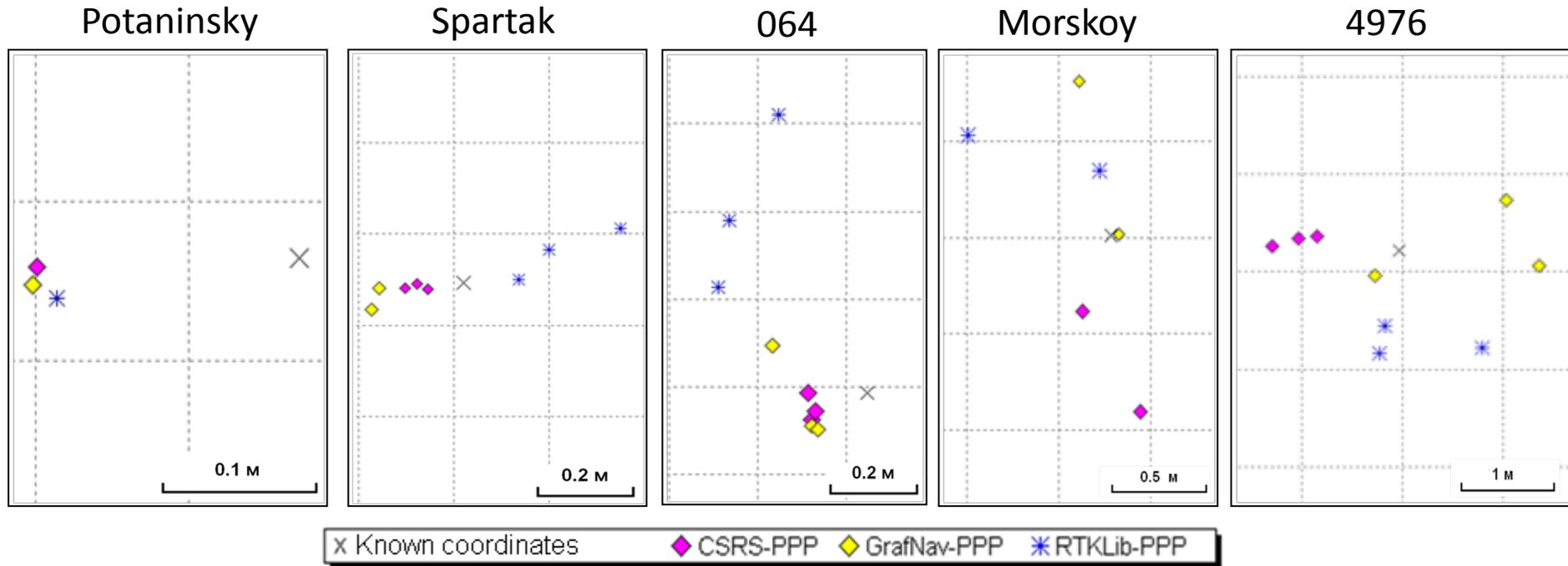
Coordinates and heights computed by RTKLib with using PPP method, have accuracy characteristics close to CSRS-PPP and GrafNav (0.1 -0.3 m in open sites and 1-2 m in leafy/pine forest). Exceptions were for short-term (10 min) measurements when RTKLib received coarser coordinates.
