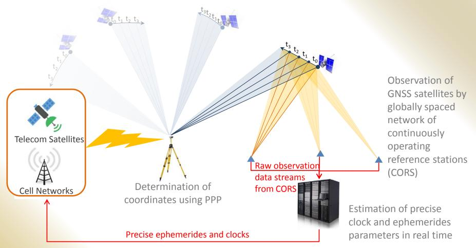
Delivery of precise ephemerides and clock parameters to the user via Internet using NTRIP protocol or via telecommunication satellite
