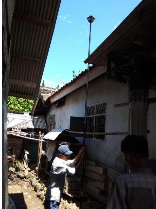
Figure 2. 4. Boundary point measurement with GPS by CLRC Team
