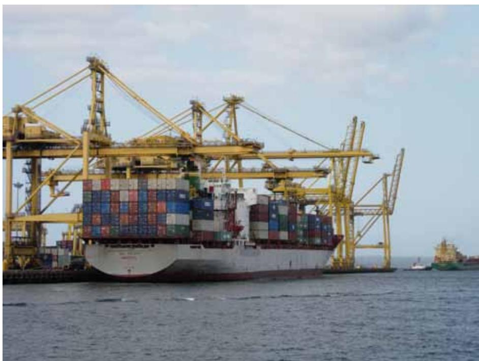
At 22,000 gross tonnes, vessels like the ANL Container Line Escort (a container ship) draw well over 10 metres of water when fully loaded. Accommodating these vessels presents a constant challenge for ports to maintain and publish up to date depth information.
