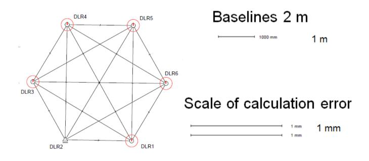
They fixed the Point DLR2 and made a free adjustment to all other points. The maximum deviation in the horizontal is 0.2 mm (red circle) and in the height is 0.1 mm (red line). I never saw a GNSS measurement with results like this before. The main reason seems to be the absolute high accuracy GNSS antenna with good multipath reduction and no near-field effects.
