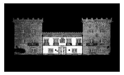
Figure 09: Result of cleaning performed on the point cloud Source: Medina, 2011
