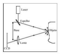
Figure 06: Scanner based on the principle of triangulation Source: BOEHLER apud Wutke, 2006
