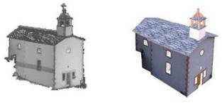
Figure 13 and 14: Point Cloud and 3D model of the Chapel "Neubrueck" SOURCE: SCHULZ & INGENSAND, 2004
