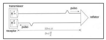
Figure 04: Principle of scanning time-of-flight (time interval) Source: MAIA, 1999
