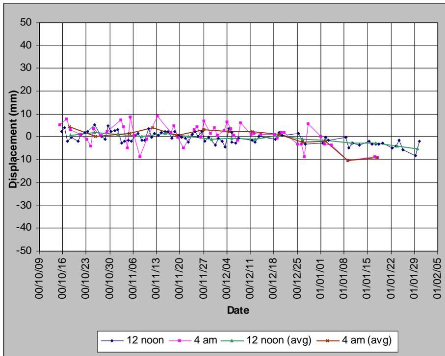
**Figure 5. Comparison of 4 am and 12 noon height determinations for point 1064.**
