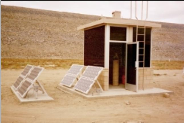
Each RTS with its computer equipment, meteorological sensors, communication radio, and power supply are housed in an observation shelter (Figure 2). Due to the remote locations of the structures, all equipment is run by DC power from solar panels located adjacent to the shelters. The solar panels charge three 25 amp batteries that were designed to supply power to all the equipment for three days without recharging.
