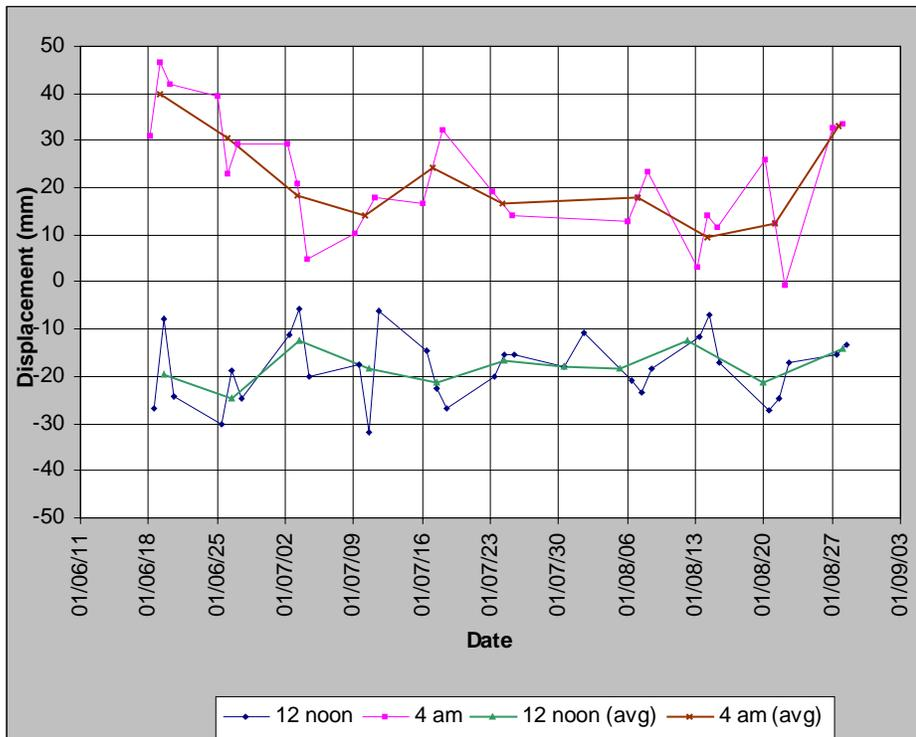
**Figure 4. Comparison of 4 am and 12 noon height determinations for point 1079.**
