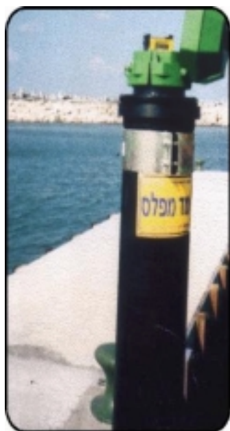
Fig.2a Float type tide gauge at the Ashqelon Marina
