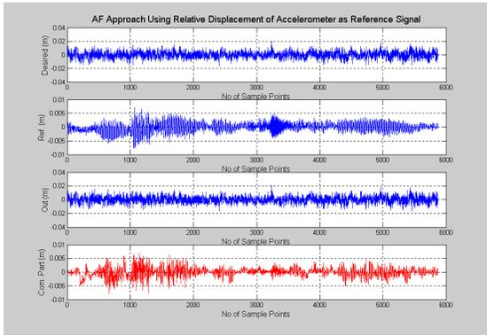
Figure 7. Accelerometer Aided AF approach
