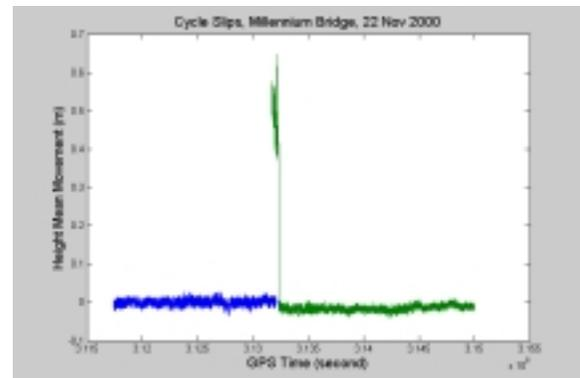
Figure 10. Cycle slips and their impact to ambiguity resolutions
