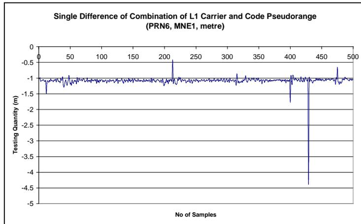
Figure 11. Single difference of L1 carrier and pseudorange
