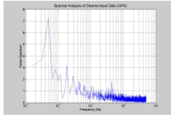
Figure 8. Spectrum of GPS data
