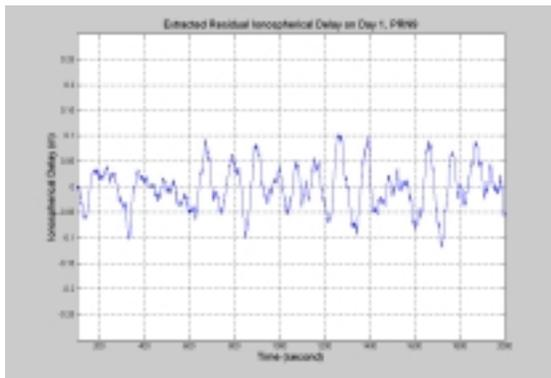
Figure 12. AF residual ionospheric delay output
