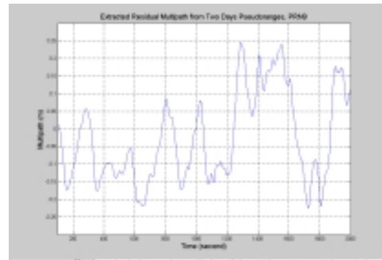
Figure 13. AF residual multipath output
