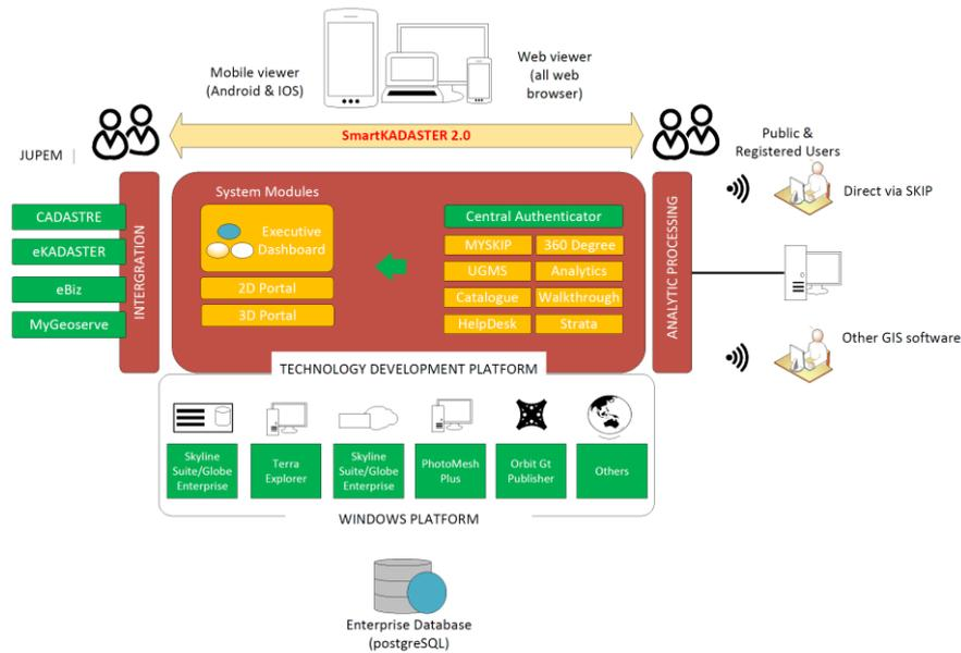
Figure 2: An Overall System Architecture of SmartKADASTER Phase 2
