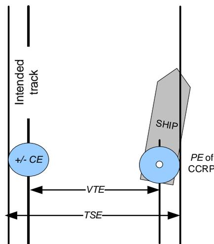
Figure 1. Contribution of GNSS position error (PE), chart error (CE), and vessel technical error (VTE) to total system error (TSE).
