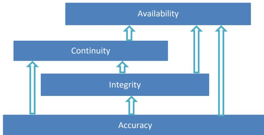
Figure 5. Dependency and hierarchy of GNSS service performance parameters in the resolution A.915(22).
