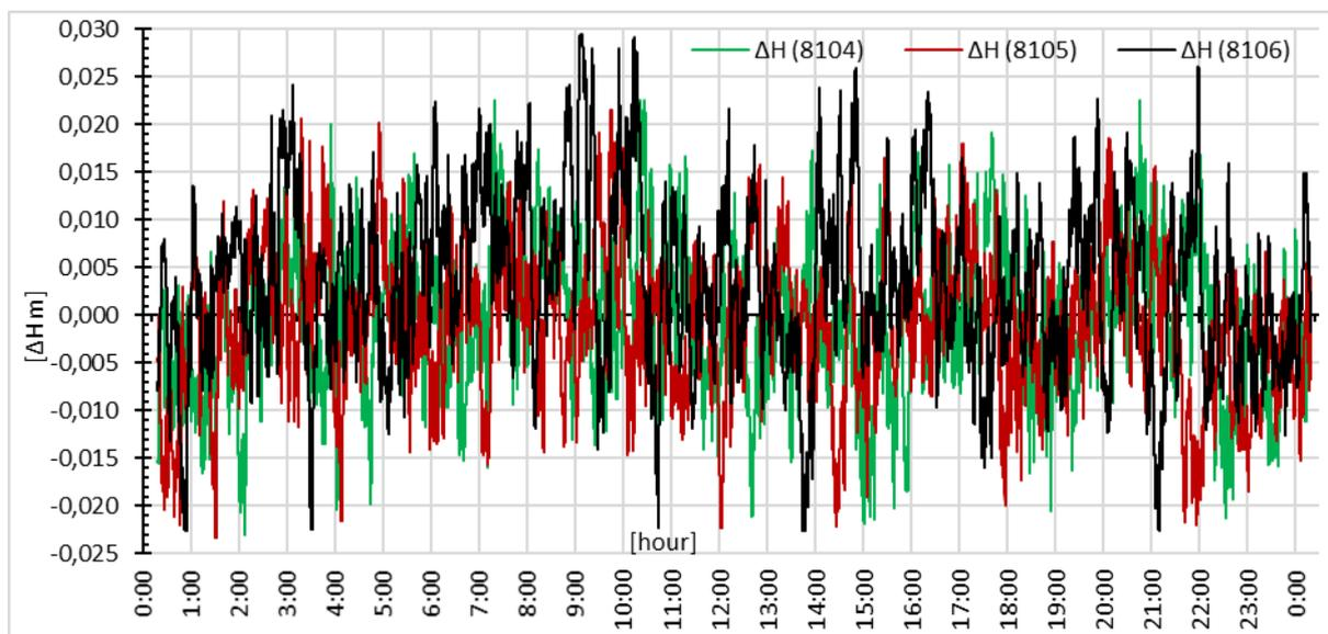
Fig. 7. Transformed time series ( $\Delta H$ ) of changes in the height component for points 8104, 8105, 8106.
