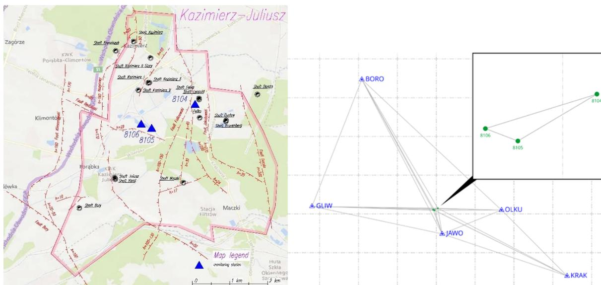
Fig. 1. Sketch of the GNSS control and monitoring network at the Kazimierz-Juliusz facility. and the location of the monitoring stations in the field
