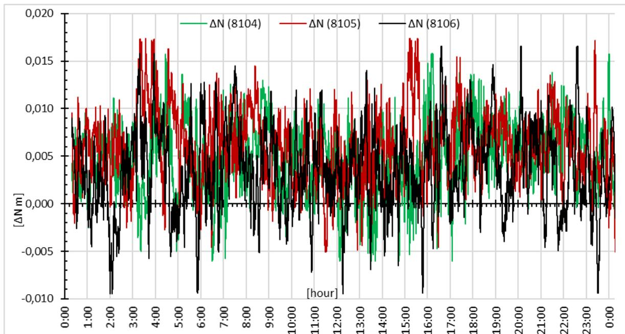
Fig. 5. Transformed time series ( $\Delta N$ ) of changes in the northern component for points 8104, 8105, 8106
