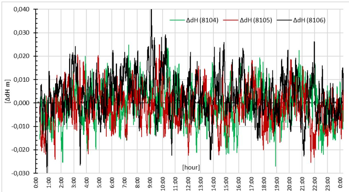
Fig. 4. Original time series ( $\Delta dH$ ) of changes in the eastern component for points 8104, 8105, 8106.
