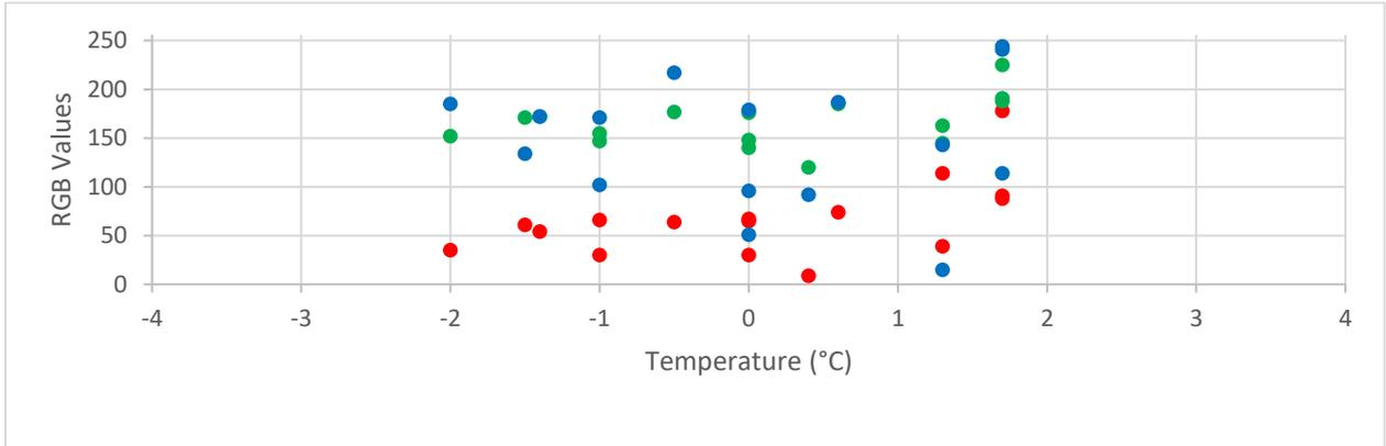
Figure 8: Plot of RGB values from the thermal orthomosaic vs temperature ground readings
