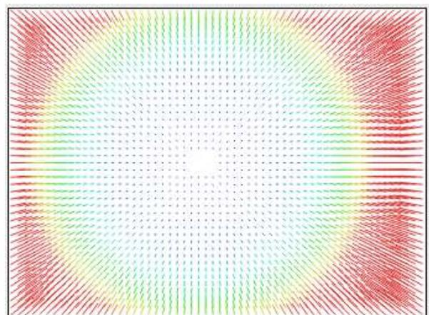
Figure 12: radial distortion from plot
