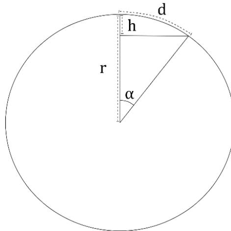
Figure 3. Height difference  $h$  due to the curvature of the Earth at distance  $d$ .  $r$  is the radius of the Earth and  $\alpha$  is the angle corresponding to  $d$ .
