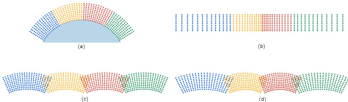
Figure 2. Different types of point cloud geometries. (a) shows how the individual scans were captured in relation to the Earth and (b), (c), and (d) are the results of different georeferencing methods. The differences in scale and the curvature of the Earth are greatly exaggerated.
